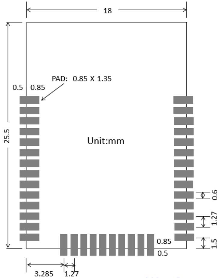
Fig. 3.3 PCB Layout for ESPC3-32
