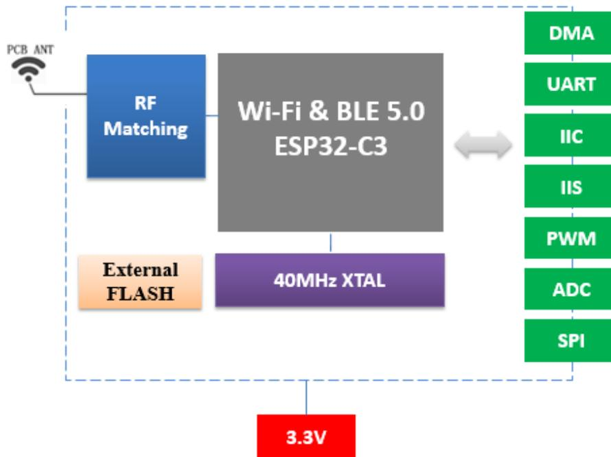
Fig.1.1 ESPC3-32 Module Structure
